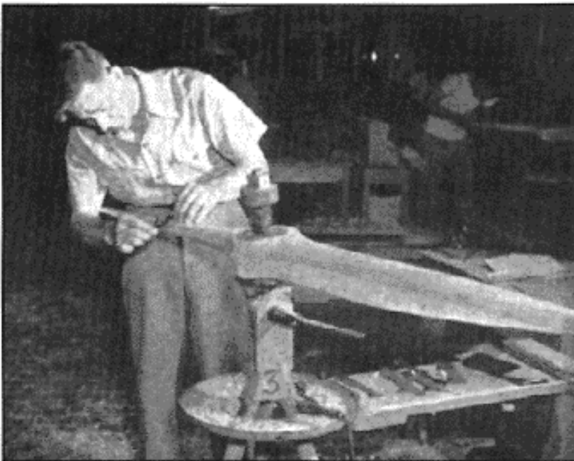
The propeller blank was clamped in it through a hole in the hub for the bushing, allowing the craftsman to tilt it in any position.
